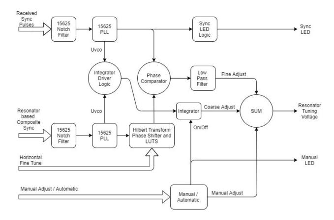
In the automatic mode (P2 fully CCW) the DSP primarily uses an integrator to adjust the resonator frequency such that the SAA1101's sync pulses match the frequency of the recovered syncpules. When the frequencies are almost aligned, the integrator is switched of and a phase comparator makes a final adjustment and maintains a phase lock. The absolute phase can be tuned using P1, allowing the horizontal alignment of the video to be adjusted.
