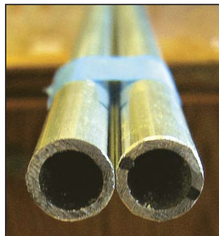
Figure 4 — Setting up two aluminum booms for marking down the middle.
