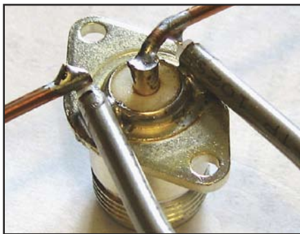
Figure 11 — Close-up of semi-rigid UT-141 coax used to make balun. It is connected to a Type N connector and the folded dipole driven element.
