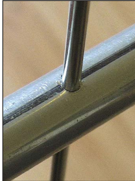
Figure 8 — Close-up of boom dimpling.
