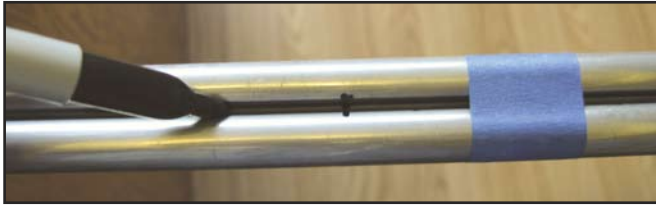
Figure 5 — Marking two aluminum booms, using each as a guide for marking the other down the middle.
