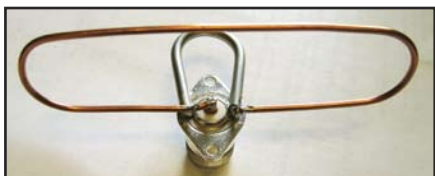
Figure 12 — Another view of the completed driven element.
