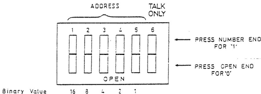
Fig. 3-13 GPIB address rocker switch bank
