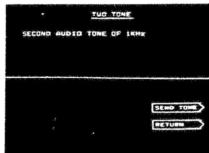
(21) Press SEND TONE and then return to TRANSMITTER TEST. 2T is shown in reverse video on the display and a 1 kHz tone in addition to the variable frequency output is connected to the AF GEN OUTPUT socket (12). The level is that set previously for the variable frequency.
