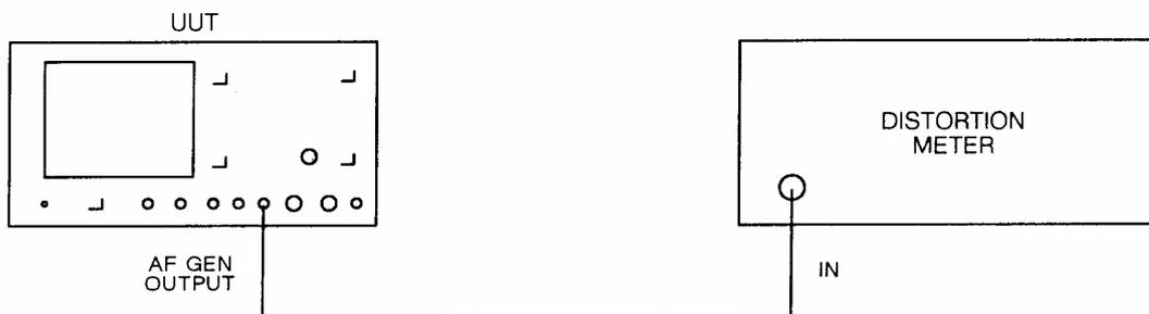
*Fig. 5-1-13 Test equipment connections for AF generator distortion performance checks*
