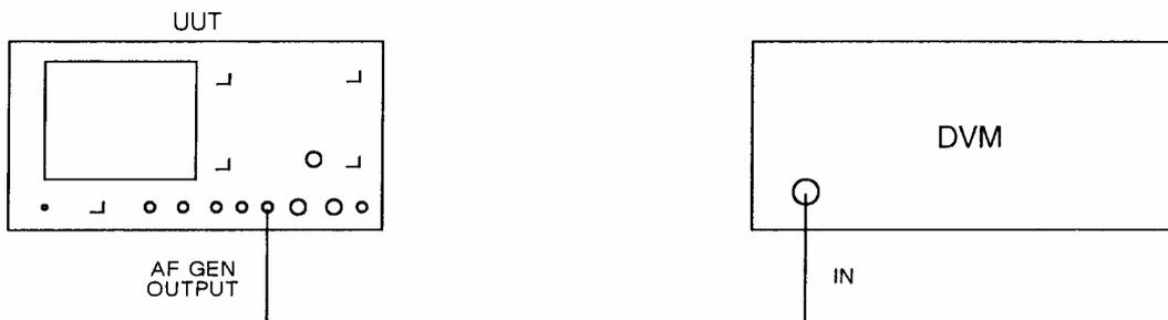
*Fig. 5-1-15 Test equipment connections for AF generator DC offset performance checks*
