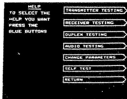
The HELP ON TESTING operating summary is then displayed – see Fig. 3-12. This includes information upon key operation, e.g. to select TRANSMITTER TEST the TX key must be pressed. But note that this is for information only: it is necessary to press the mode key arrowed by RETURN twice (once to return to the HELP menu and once to return to the operating mode) before pressing the designated key.
