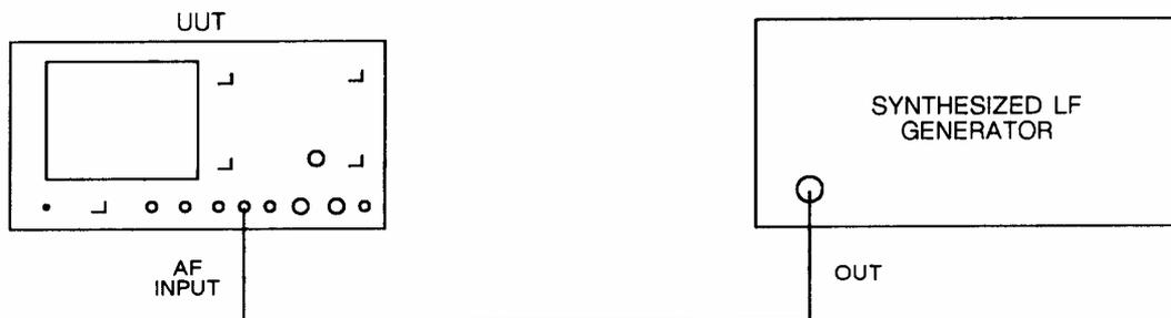
Fig. 5-2-6 Test equipment connections for adjusting R305 and R314 on AB5/I
