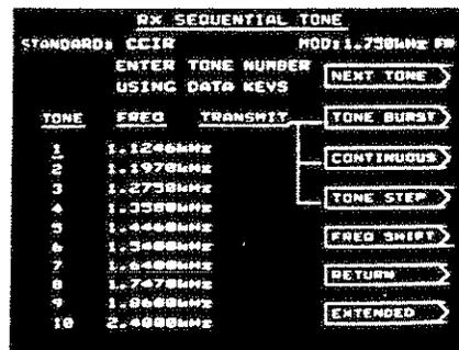
(14) Enter the tone number using the keypad (6) and press the key which is arrowed by NEXT TONE to terminate the entry. This causes the frequency to be displayed against the entered tone number and moves the cursor down ready for the next entry.
