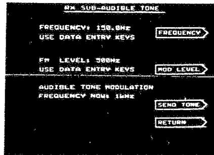
(7) Press the key which is arrowed by FREQUENCY and set the second. variable frequency using the keypad (6), ending with the frequency terminator (7).
