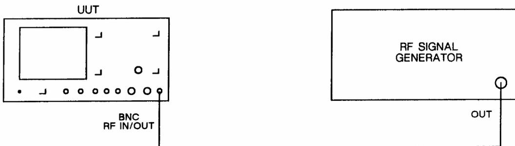
Fig. 5-1-28 Test equipment connections for 2955R level accuracy check
