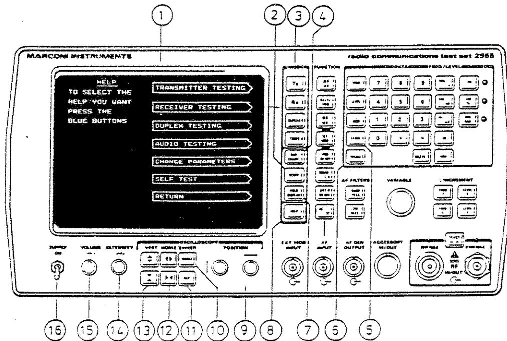
Fig. 3-1 Front panel
