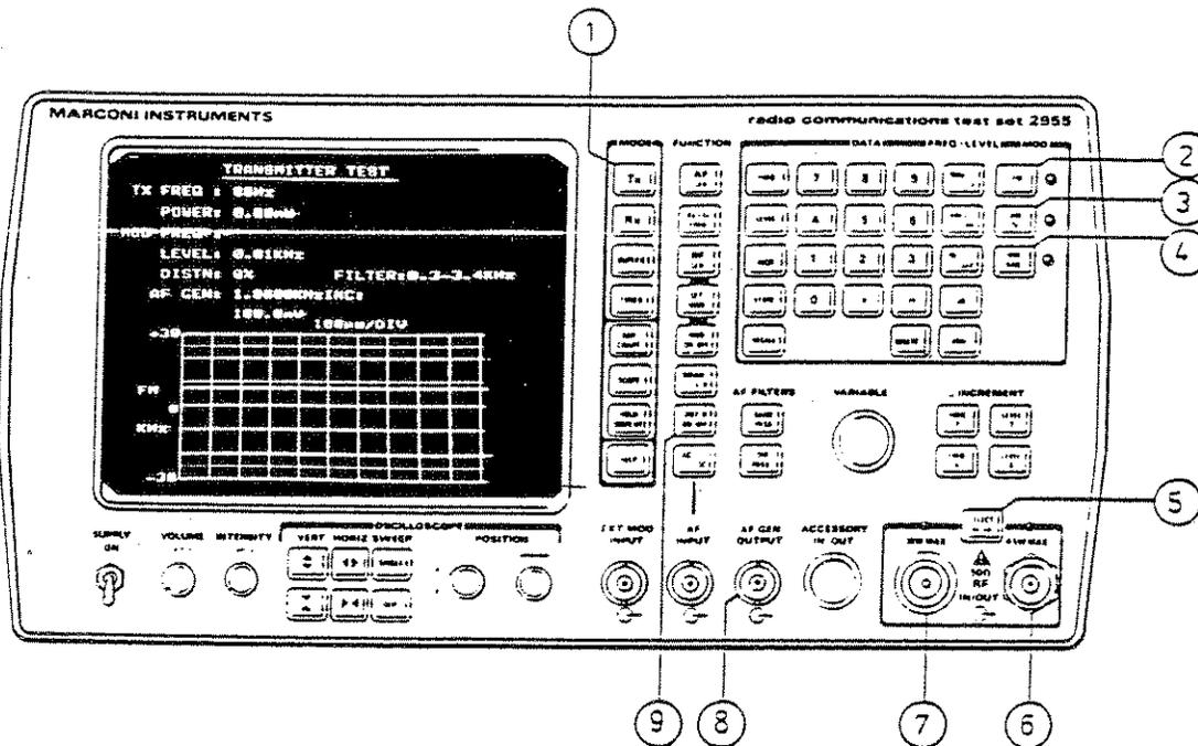
Fig. 3-6 Distortion meter (TX) controls and connectors
